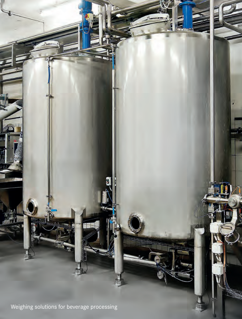
Load cells for mobile hygienic vessels
