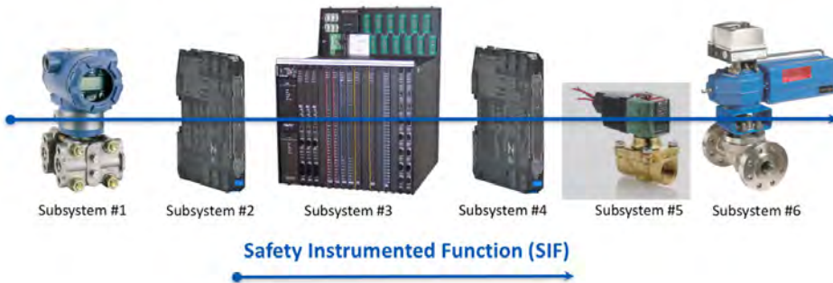
Figure 88, Example of a simple 1oo1 SIF
