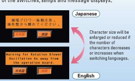
Extended alarm functions for reduced labor thanks to added enhanced functions
