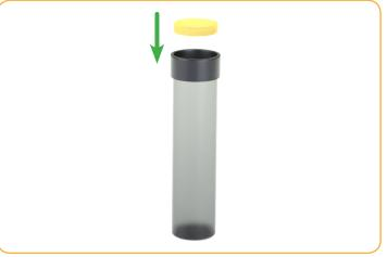
Saturate the sponge wafer (use approximately 10 mL of water) and place it in the bottom of the calibration chamber.
