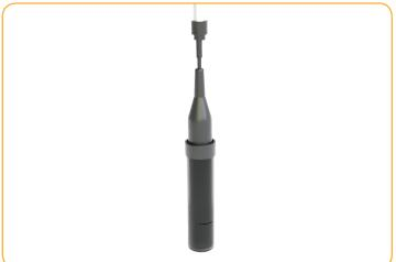
Remove the water-saturated sponge from the calibration chamber and fill the chamber to the fill line with approximately 60 mL of fresh sodium sulfite solution.
