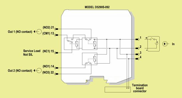
Relay contact shown in de-energized position. Terminals 13-21 and 14-22 are open; terminal 13-15 is closed.
