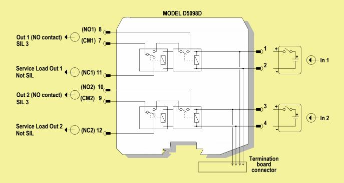
Relay contacts shown in de-energized position. Terminals 7-8 and 9-10 are open; terminals 7-11 and 9-12 are closed.
