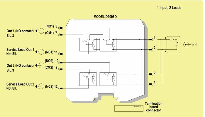
Relay contacts shown in de-energized position. Terminals 7-8 and 9-10 are open; terminals 7-11 and 9-12 are closed.
