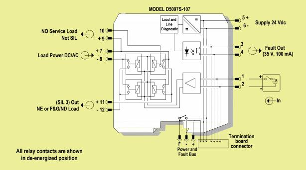
To prevent relay contacts from damaging, connect an external protection (fuse or similar), chosen according to the relay breaking capacity diagram.
