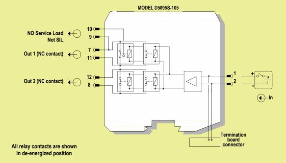
To prevent relay contacts from damaging, connect an external protection (fuse or similar), chosen according to the relay breaking capacity diagram.
