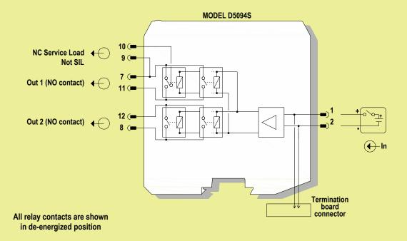
To prevent relay contacts from damaging, connect an external protection (fuse or similar), chosen according to the relay breaking capacity diagram.
