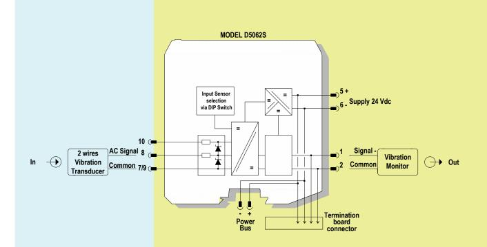
Input configuration selection via internal Dip-Switch
