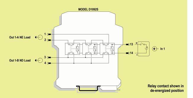
To prevent relay contacts from damaging, connect an external protection (fuse or similar), chosen according to the relay breaking capacity diagram.
