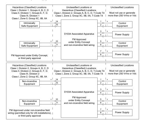
Non-incendive field wiring is not recognized by the Canadian Electrical Code, installation is permitted in the US only.
