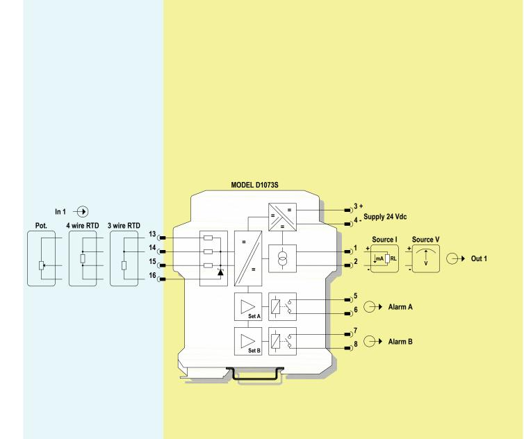
For SIL applications, alarm contacts must be used in series with equal configuration. Relay contact shown in de-energized position
