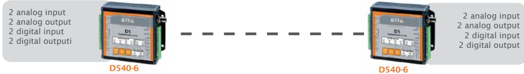
Point-to point wireless connection mirror type allows to mirroring the I/O status of each unit.
