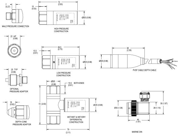
NOTES: [1] ALL DIMENSIONS ARE IN MILLIMETRES (INCHES) [2] HIGH PRESSURE IS >70 BAR
