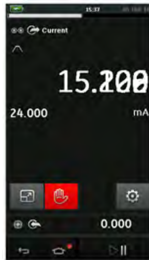
RAMP automatic cycle
